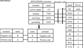
Fig. 3-12 RS485 communication wiring
