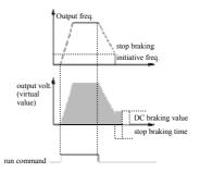
Fig.6-8 Dec stop+DC braking
