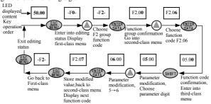
Fig.4-7 example for parameter setting and modification
