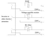
Fig.3-17 installation demand for electromagnetic on-off device
