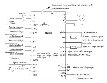
Fig. 3-6 basic wiring diagram
