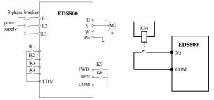
Fig.6-25 multi-step speed run
