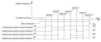
Fig.6-24 multi-step speed run
