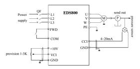
Fig.6-13 built-in PID analog feedback control system graph
