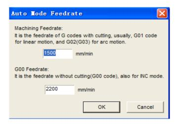
When the system in the manual way, the pop-uping dialog box uses to establishing the velocity of the manual movement, like the chart shows
