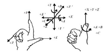
In the milling class engine bed, the direction of the engine bed 's coordinate axis is decided by both the type of the engine bed and the layout of each parts, speaking of the milling machine, the basic coordinate axis is X, Y, Z:
