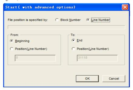
In the dialog box, the manager set the starting position and the ending position of the procedure in executing process, then clicks the "start" button, the engine bed carries out the segment assigned in whole processing procedure according to yours request.
