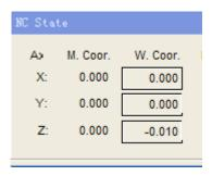
The system has provided the convenient setting and the method of modify the workpiece origin, setting the current point to the workpiece origin, as well as the relative position of the click axis clears zero, Only must moving the cursor to this axis coordinates show area, then clicks the mouse's left key, thus may see that this axis's coordinates become 0. If you want the current positions of 3 axes are established to 0 completely, only clicks in each coordinates area.
